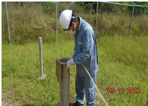
Up Gradient Monitoring Well
