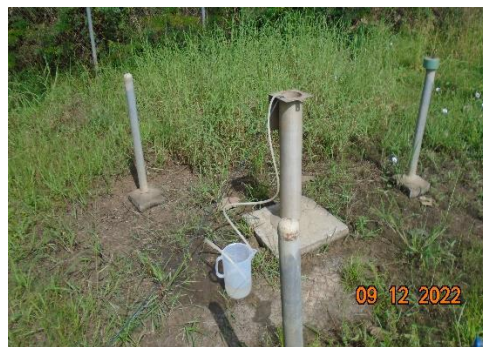
Down Gradient Monitoring Well
